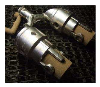
**Nanocomp BC11** is a conductive coating providing good mellt flow properties and rapid solidification for many castings. This coating provides productive conditions for castings non-sensitive to cracks.
